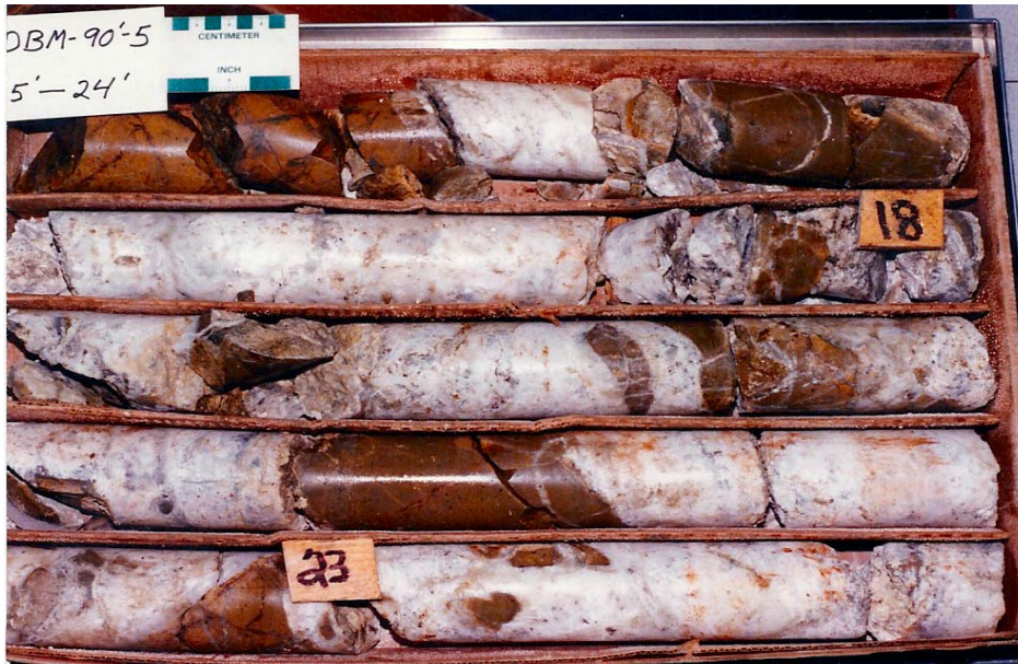
Figure 13.3: Core From Degerstrom Hole 90-5 (14.5–24 ft)
