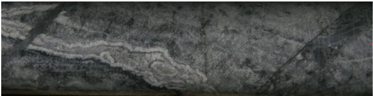
Figure 7-22 Breccia dykes (left and right end of photos) with chaotic breccia inside dykes, cross-cuts colloform banded iron-carbonate vein
