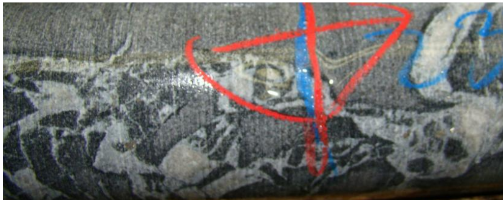
Figure 7-11 Fe-carbonate breccia in crystal tuff unit in hangingwall
