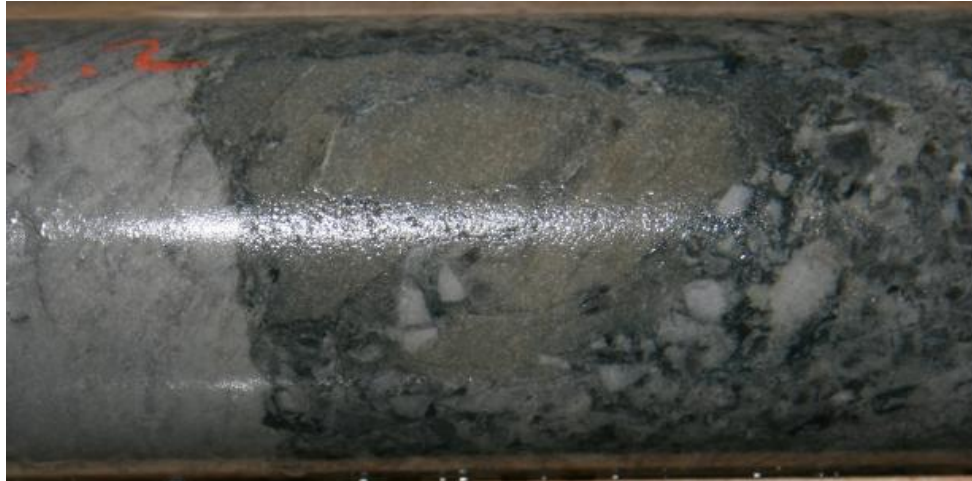
Figure 7-20 Chaotic breccia with multiple clast types. Sericitic fragment in centre of photo is crystal tuff
