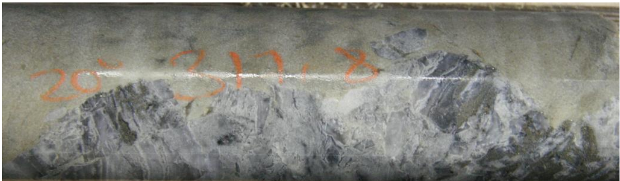
Figure 7-21 Clast rotated breccia. Note: crystal tuff unit (near top of photo) cuts breccia fragments. This is part of a larger interval of crystal tuff which may be a large fragment
