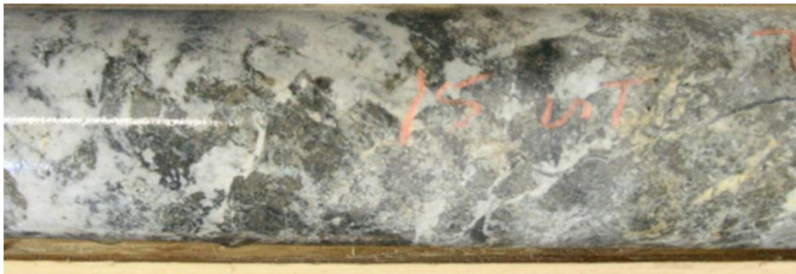
Figure 7-13 Partial replacement of fragments with Magnetite
