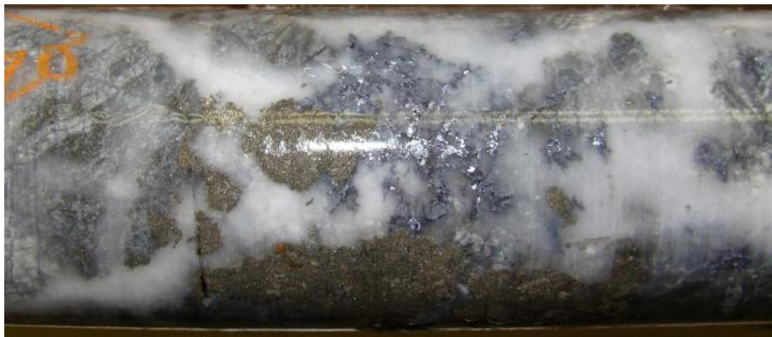
Figure 7-14 Silica cement with pyrite and galena. Fragments are partially replaced by pyrite
