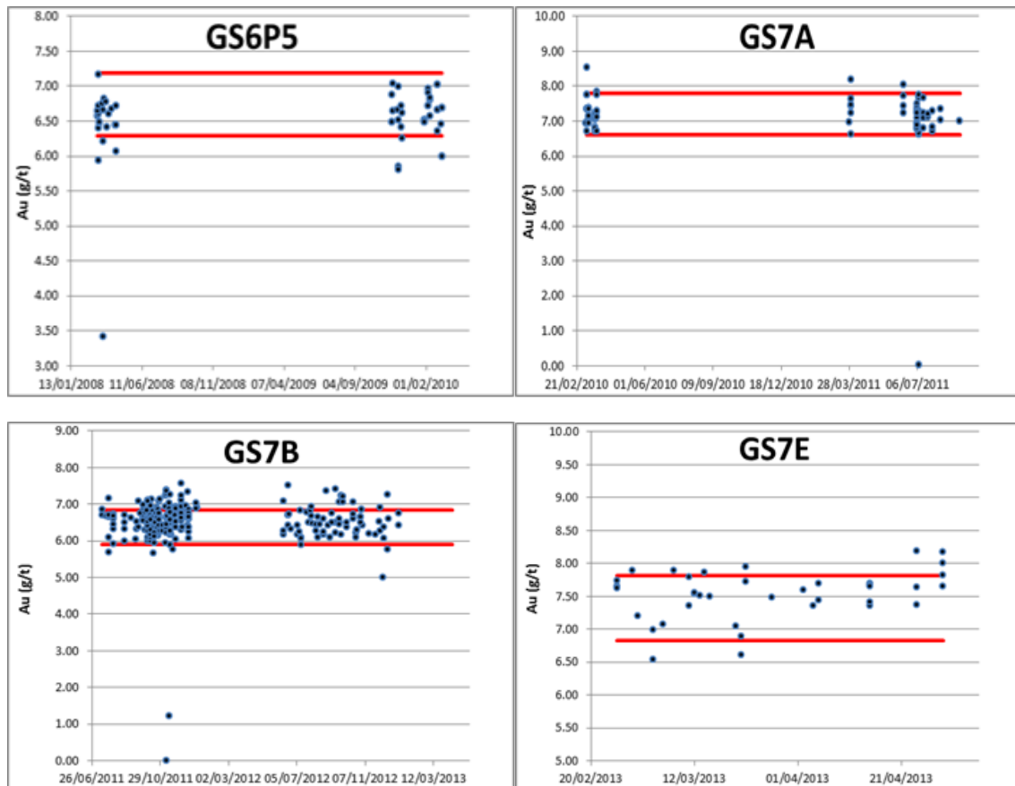
Figure 12-2 Results of the Individual Standards Used and Relation to Anticipated Value Range (between red lines of 2SD)
