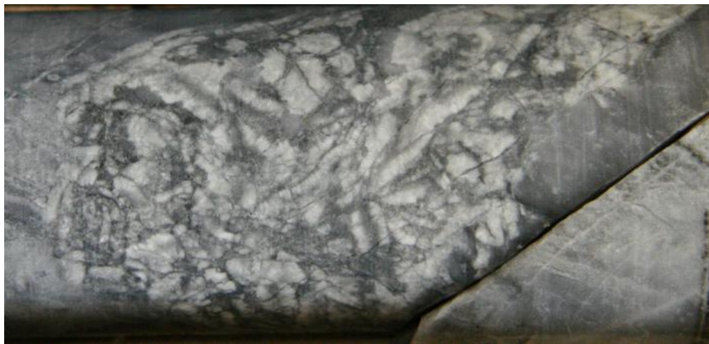
Figure 7-17 Iron-carbonate vein fragments (and possible coxcomb textures)
