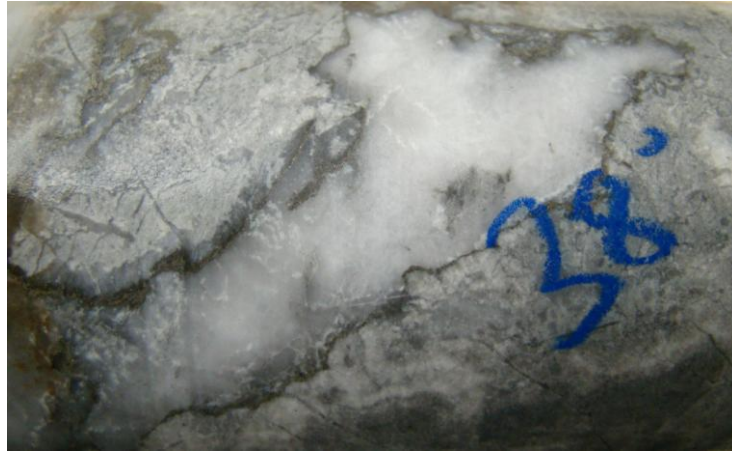
Figure 7-12 Pyrite rims on silica. Partial replacement rims on fragments. This texture is very common throughout the breccia and in areas of "laminated cherts/tuff"
