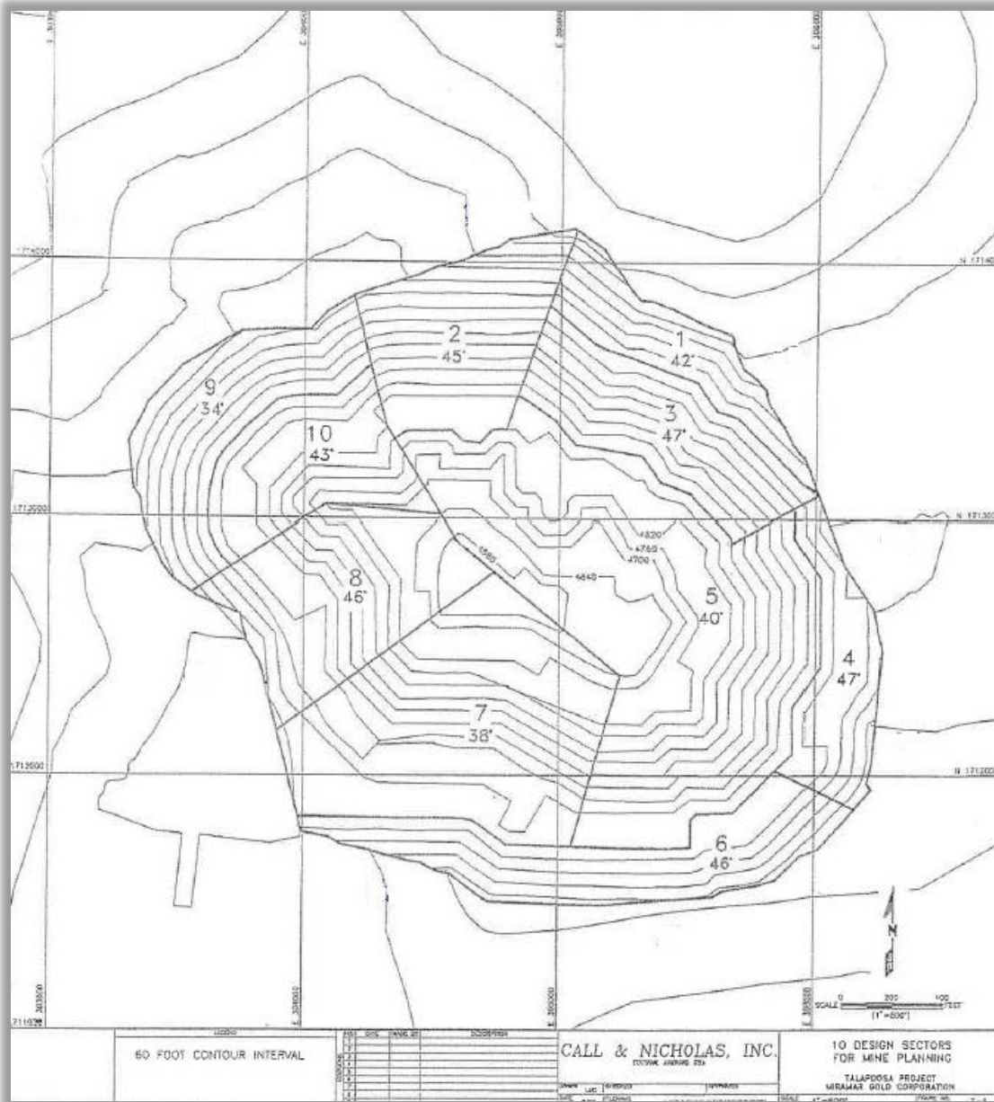
Figure 16.1 – Design Sectors and Slope Angles for Mine Planning (Calls & Nicholas, Inc., 1995)
