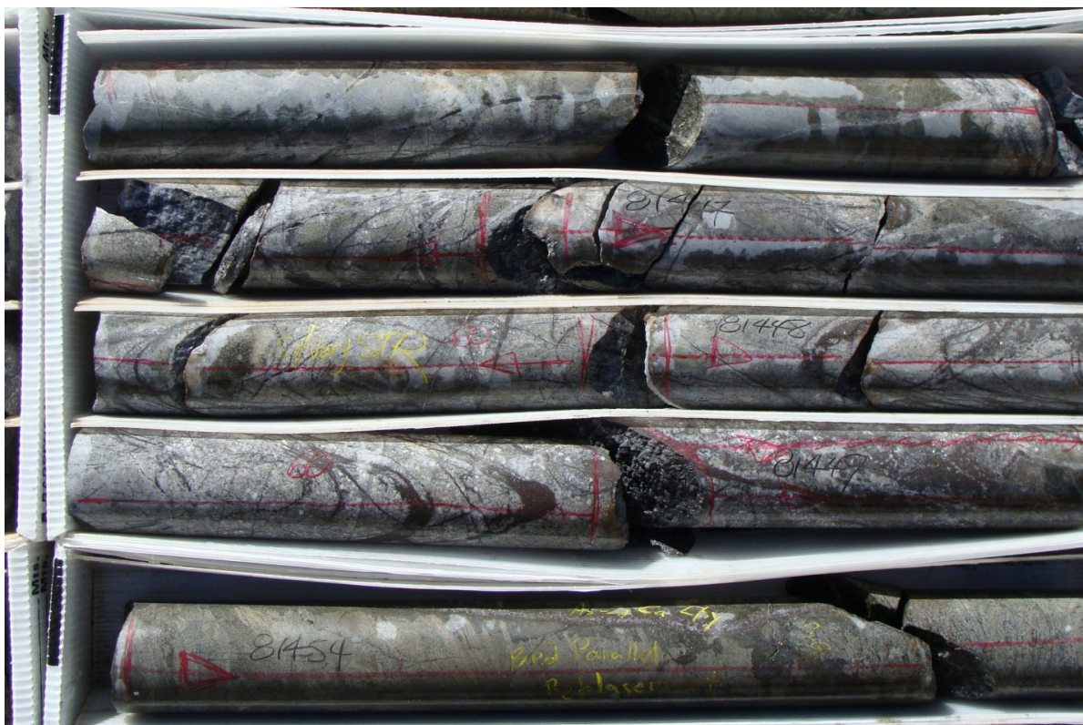
Figure 15: Photo of the EndoSkarn Zone (Fernandez) comprising stockwork sulphide mineralization hosted in the Wall-rock Unit ; ddh SD-12-50 W2.
