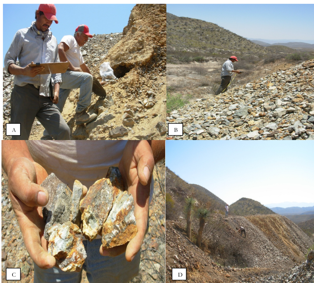
Figure 107: Clockwise: A) Technicians recording sample information. B) Measuring distances between samples at the La Cruz-Adelaidos pile. C) Waste material typically sampled from the La Cruz-Adelaidos pile. D) Technicians sampling the sides of the La Cruz-West pile.
