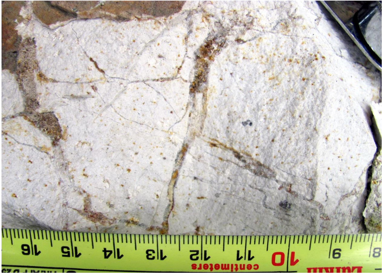
Figure 7-4 Poorly to moderately developed stockwork of millimeter-scale quartz and iron oxide veining/fracture-filling in rhyolite quartz-eye porphyry (UTM 482717E, 2284684N). Soltoro grab sample 371717 returned 3.511 g/t Au. Howe verification sample N935869 returned 1.84 g/t Au over 1 metre.
