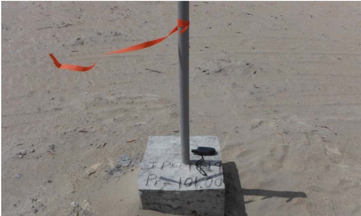
Figure 12-2: Example Drill Hole Monument for JPQ-14-19
