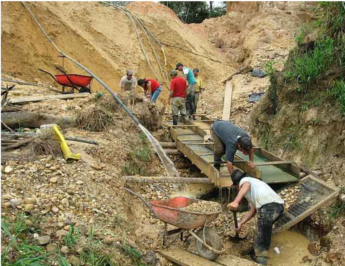
Figure 20. Sluice box cleaning at Patuca, an artisanal gold mine in the southern Cordillera de Cutucú. Photo by Keith Barron, 2008.
