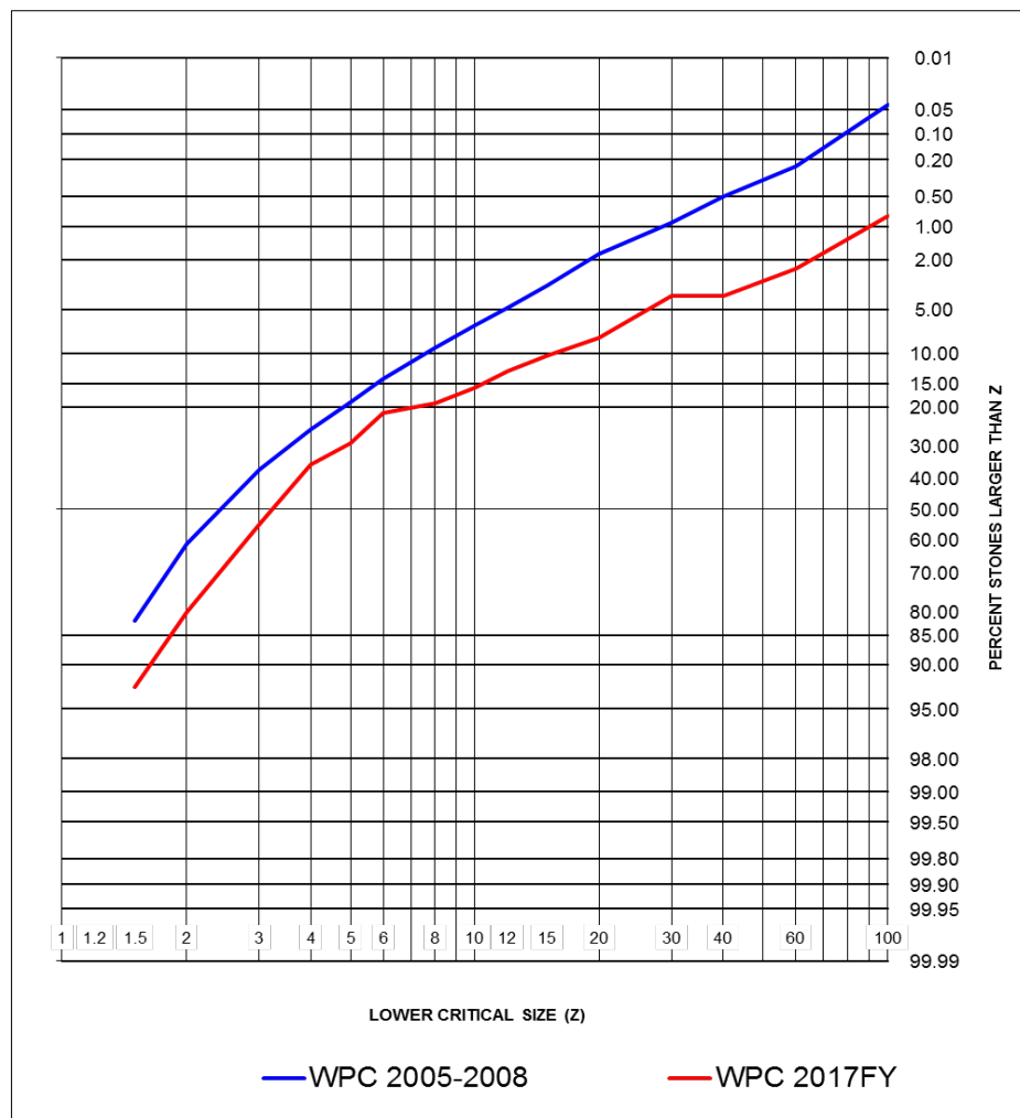
Figure 8.7 SFD of diamonds from Wouterspan 2016/2017 programme compared with the 2005-2008 programme
