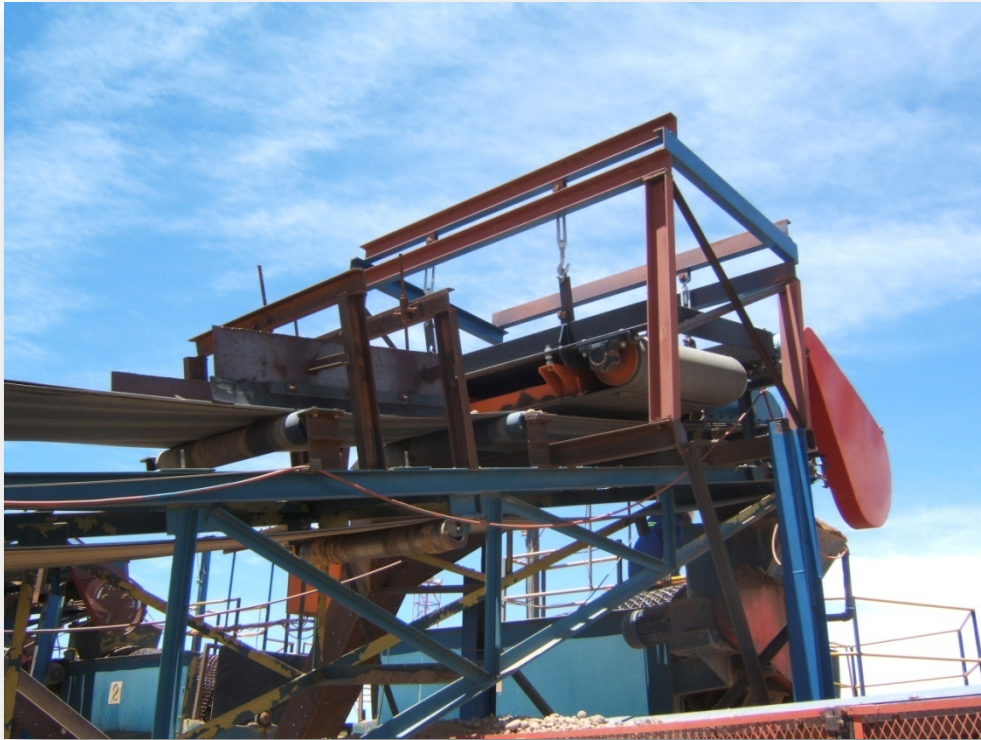
Plate 8.1 Magnet suspended above plant feed belt to separate out the BIF clasts
