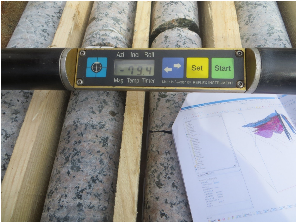
FIGURE 10-2 REFLEX EZ-SHOT INSTRUMENT USED IN DOWNHOLE SURVEYING
