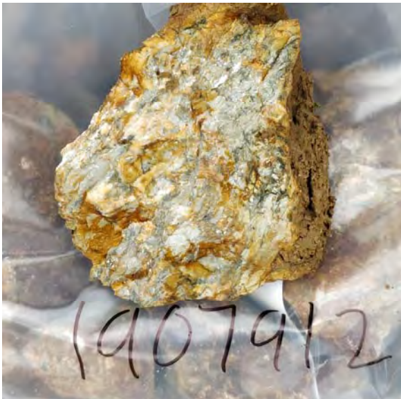
Figure 30: Sample 1907912 Outcrop approximately 100 metres south of Golden Culvert main showing area; silicified phyllite and quartz veining; 4% sulphides; assay of 7.16gpt Au.
