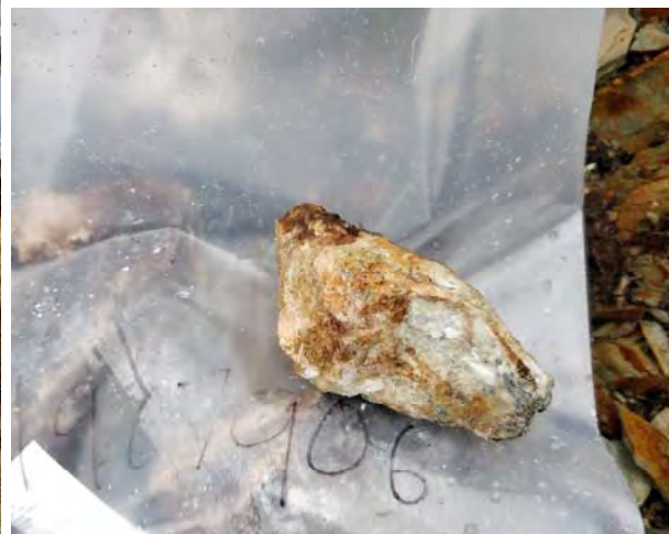
Figure 28: Sample 1907906 Quartz vein in Golden Culvert main showing striking 305°; 1% euhedral pyrite; assay of 13.38gpt Au.
