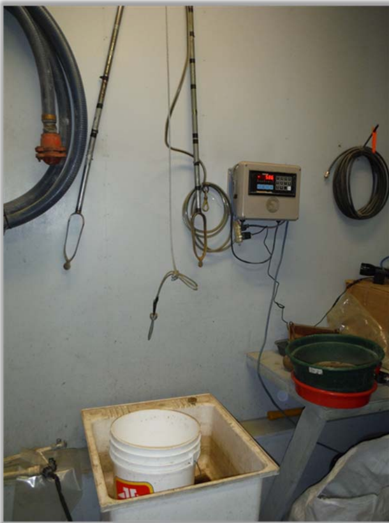
Figure 14.11 Specific Gravity Scale in Core Logging Facility
