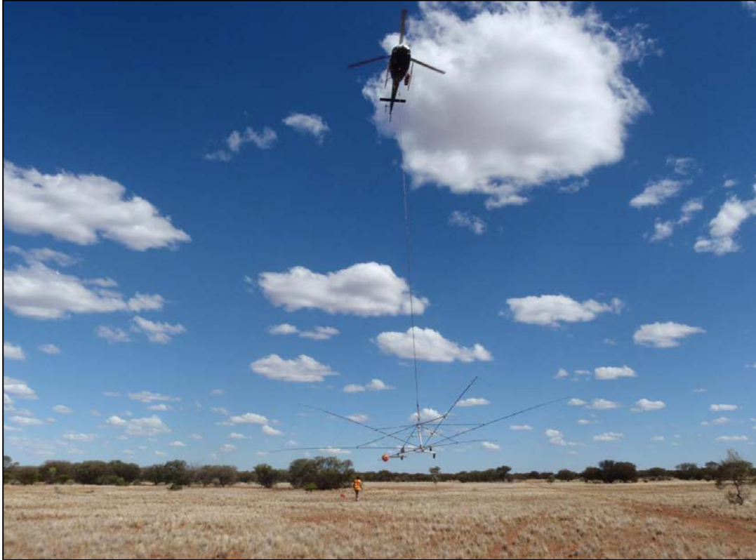
Figure 25: Photo of aerial XTEM survey equipment
