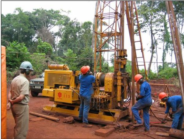
Large diameter coring operations – pulling the core barrel at FM 78
