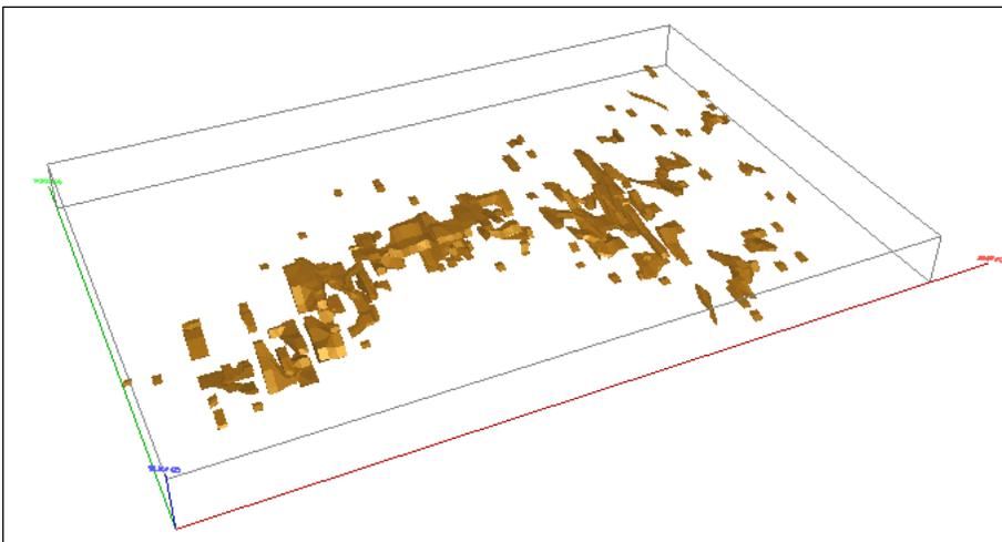
**Figure 14.5 V2 along block model 621937.5 mE (column 30) – percentage waste incorporated into blocks**
