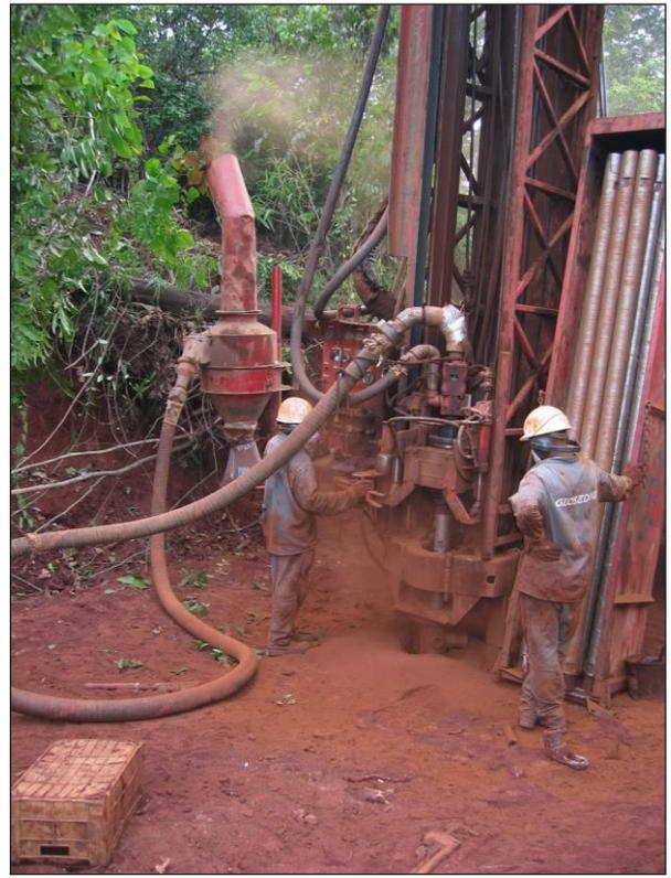
Infill RC operations – Prospector W750 articulated rig at V1 LT725W
