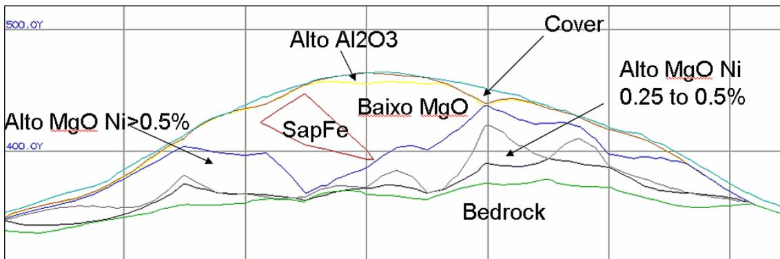
Note: This is a screen snapshot from Gemcom software. Grid spacing is 100 m. "400Y" is 400 m elevation.
