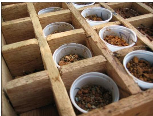
Storage of RC chips for reference – lid was removed from box
