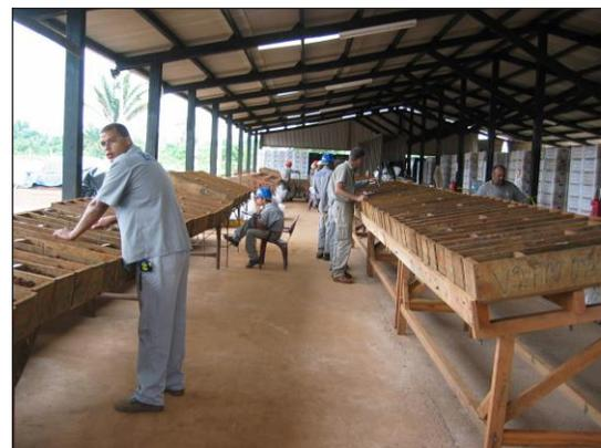
Logging and sampling of large diameter cores
