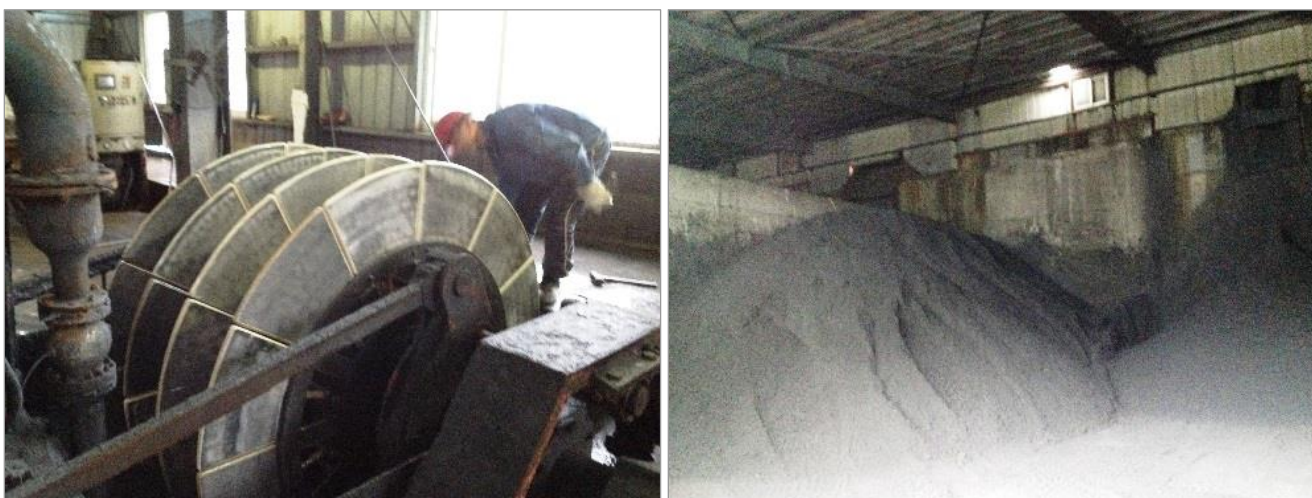
Figure 17.7 Disc filters and zinc concentrate shed
