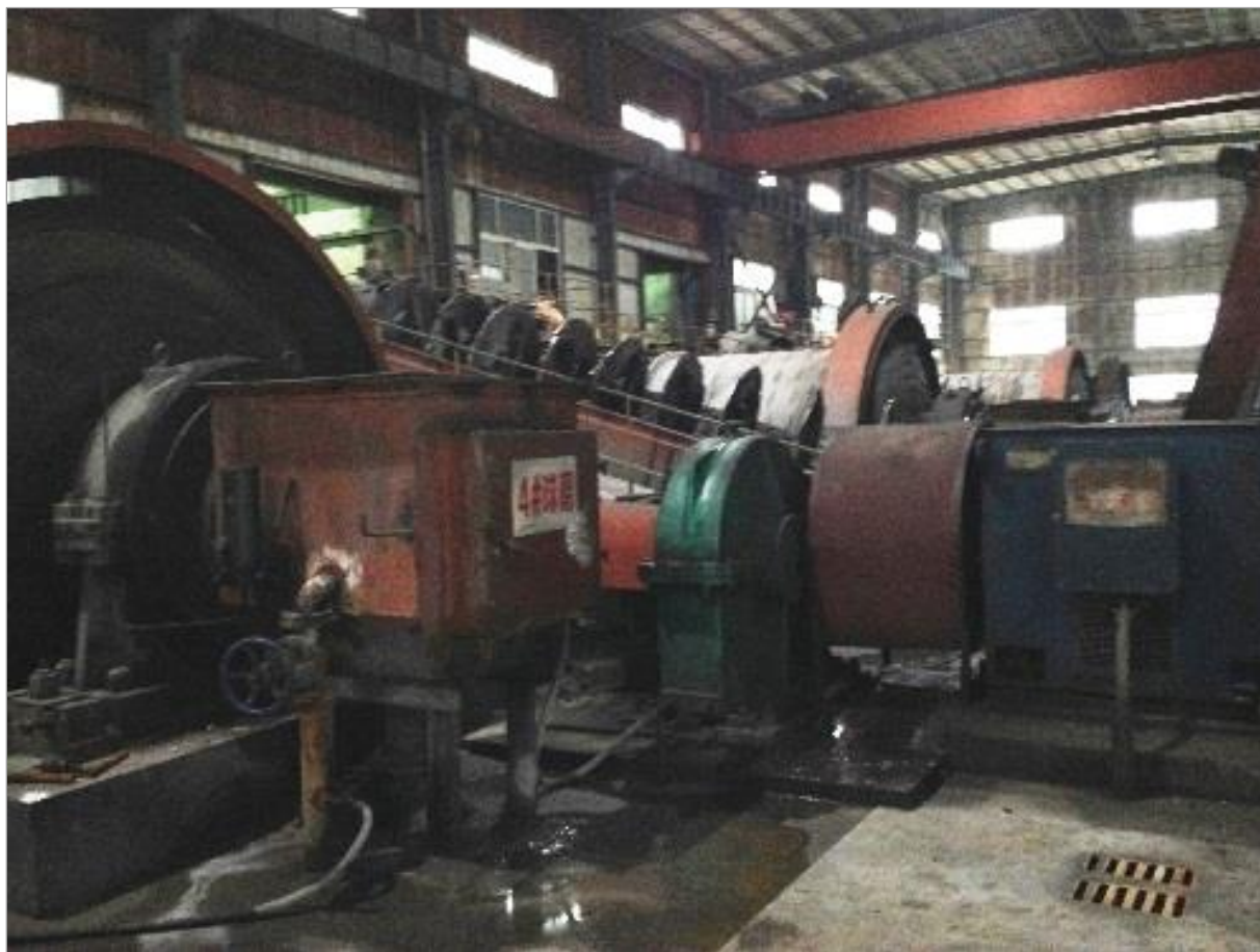
Figure 17.4 Grinding mills and spiral classifier
