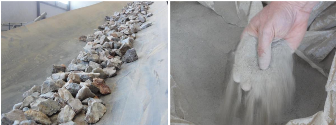
Figure13.2. Sulphide ore before milling and after a single pass of milling in the multi-shaft EDS mill.
