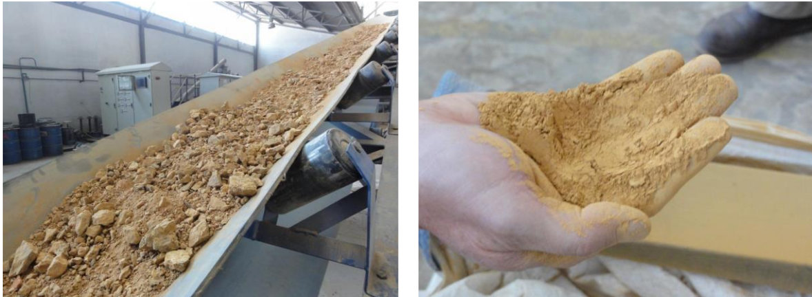
Figure13.1. Oxide ore before milling and after a single pass of milling in the multi-shaft EDS mill.
